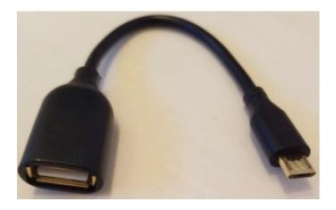
Notice the "female" connection on the left side view. This is where the "male" connection on the bar code scanner will go. There is no electronics in these adapters, the are simply reducing the connection from the large USB to the small micro plug, so they are rather inexpensive. Here's our total setup:
