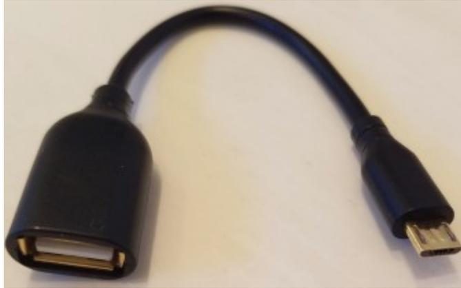
Notice the "female" connection on the left side view. This is where the "male" connection on the bar code scanner will go. There are no electronics in these adapters, they simply reduce the connection from the large USB to the small micro plug, so they are rather inexpensive. Here's our total setup:
